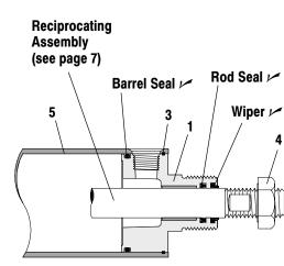
Moderately lubricate barrel I.D. and all seals with Shell Darina EP Grade #2 Grease.
